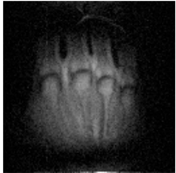
Fig. 13. Coronal spin echo image of hand acquired at 0.01 T with the litz receive coil at 77 K (imaging parameters as for Fig. 12 except TR = 400 ms).
